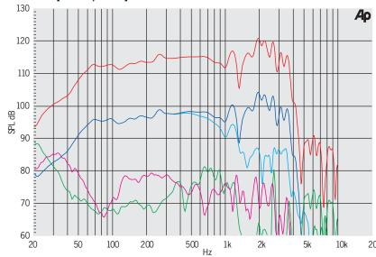
Data measured using swept sine wave input on an open baffle of dimensions 2.5 x 3.7 metres with a microphone distance of 1 metre.
