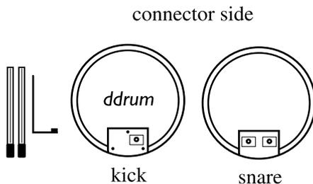
You need to assemble the L-shaped pedal attachment and the two chrome legs to the kick pad. The necessary nuts, bolts and washers are located within the package that contains the legs. The only tool needed is your drum key. The pedal attachment has three holes for the bolts and one square cut-out, for the connector output. The shorter part of the L should point in the direction towards your playing position.
