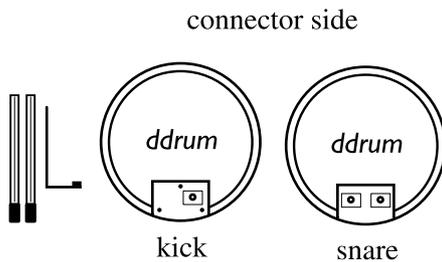
You need to assemble the L-shaped pedal attachment and the two chrome legs to the kick pad. The necessary nuts, bolts and washers are located within the package that contains the legs. The only tool needed is your drum key. The pedal attachment has three holes for the bolts and one square cut-out, for the connector output. The shorter part of the L should point in the direction towards your playing position.
