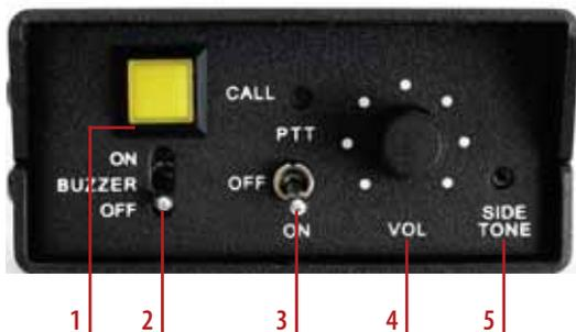
**CALL**-button (1), with light indicator. Below is the buzzer ON/OFF switch (2), to generate an acoustical call buzz. In the middle of the panel is the 3-position microphone switch: **ON** (permanently), **PTT** = Push To Talk and **OFF** (3). Finally the volume control for the earphone (4) and the **SIDE-TONE-control** (5) for setting the cue volume of your own microphone. For all these controls the same hints apply as outlined for the master station MS-200.
